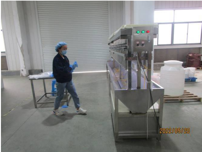
Water leakage test
