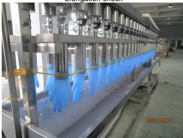
Water leakage test
